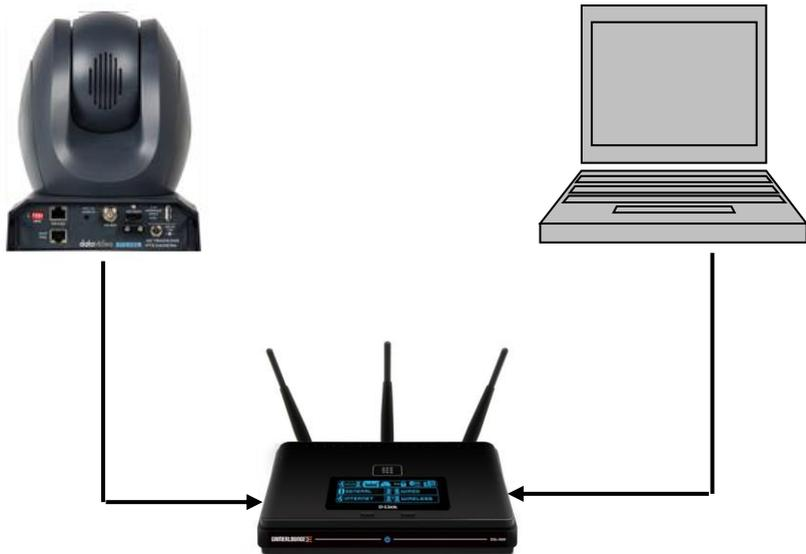
In order to enable the DHCP mode of the camera, please select “Dynamic IP Address” from the “IP Configuration Type” drop-down menu for assigning a dynamic IP address to PTC-305NDI by the router. After that, please click the “**Apply**” button to save the new settings and then please reboot the PTC-305NDI.
