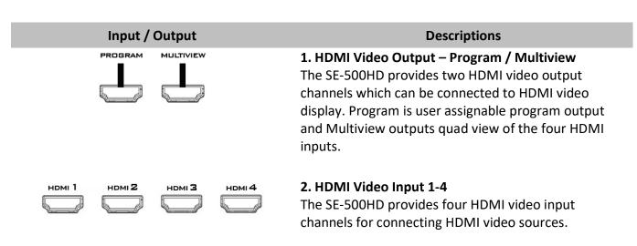
Note: A mix of combinations of different input resolutions can be connected to the HDMI video inputs. Listed as follows are the available resolutions supported.
