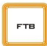
The **FTB** button (Fade To Black) fades the current video program source to black. When pressed again it acts in reverse from complete black to the currently selected program video source. To set the transition time, open the OSD menu, then the Start menu, and modify the FTB value accordingly.
