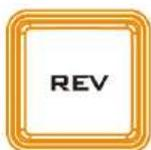
When the **REV** Button is **OFF** the selected WIPE or DVE transition will operate in its default direction only. When the **REV** Button is **ON** then the selected transition will operate in the reverse direction.
