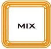
The **MIX** button is selected when a dissolve or fade transition between the selected Program and Preset sources is required. This **MIX** transition is produced by then moving the **T-Bar** manually or by pressing the **AUTO** button. To configure the mix transition time, open the OSD menu, then the **Start** menu, and modify the **M/E** value accordingly.
