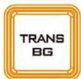
Turning on the **TRANS BG** button allows you to activate the MIX, WIPE or Stinger transition with the background image/video.
