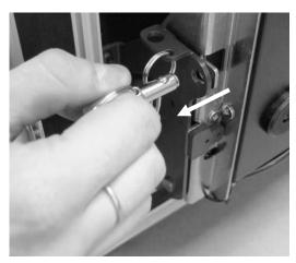
The bolts can then be stored on each hinge bracket before lowering the Control Panel Keyboard.
